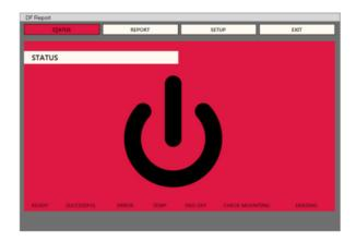
If you have installed the report and certificate kit, optical sensors will identify the status of the degausser and when ready you can use the remote control to start the erase process. The software controls the communication from the degausser through the reporting hardware kit to the reporting control centre where the operator can create, save or edit reports. These reports can be printed as a certificate or uploaded to the Blancco Management Console.
